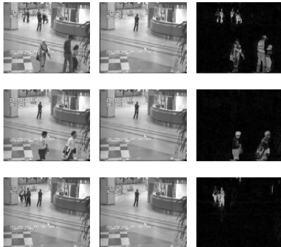
Figure: Surveillance video as a rank-sparse model: Left = low-rank (middle) + sparse (right)
